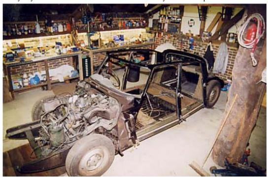
No new metal was needed in the roof rails. The roof rails were taken back to bare metal and re-painted again using a 2-pack etching primer. The opportunity was also taken of rerouting the aerial cable along a roof rail, down by the 'C' post, through the sill and up the 'A' post to the radio. Originally the cable ran up the windscreen pillar and could be seen.
