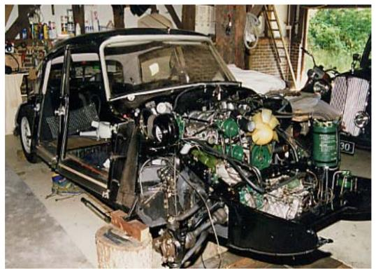
The engine gearbox assembly back in the restored chassis punt and ancilliaries plus hydraulic units being re-fitted. Note that the car is supported each side by two tree buts under the re-inforcing point. Underneath the car is a full length pit, which makes fitting things like the exhaust system so much easier. In the background is my 1946 Rover P2 14hp.
