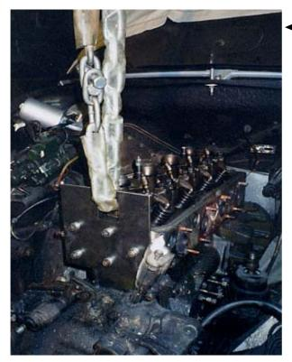
To reduce the weight as much as possible; I was working single handed - all engine ancilliaries were removed before the engine/gearbox assembly was removed from the car.
