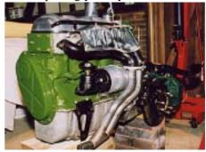
The restored engine waiting to go back in the car. The twin exhaust downpipes are now stainless steel; as are most fasteners used throughout the restoration.
