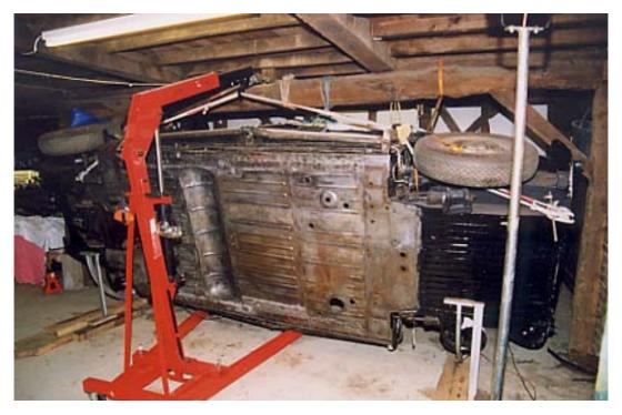
Welding on the floor pan now complete and painting underway, from the rear working towards the front. A 2-pack epoxy etching primer was used, followed by a coat of chassis black and finished with a sprayed coating of a flexible wax based underseal. All cavities were saturated with Waxoyle. The vertical aluminium tube in the foreground, is a portable Halogen floodlight.
