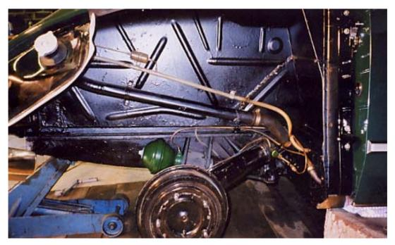
The restored offside rear wheel arch. The 'book' says there is 80 feet of hydraulic piping in the DS. I used just over 100 feet - but that included the learning curve of both forming nipples and bending the pipework neatly. All pipework is now in cupro-nickel and will not rust.
