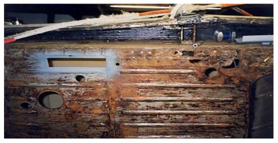
The corroded floor pan. Rusted parts were cut out and dealt with in sections. By welding in new metal in lengths of not more than a foot long, panel distortion was avoided. After cutting out the rust, the panel edges were primed with a Zinc rich weld-through primer, before new 18 gauge metal was Mig welded in. At the top of the picture you can just see the white tow rope to which the engine crane was attached.
