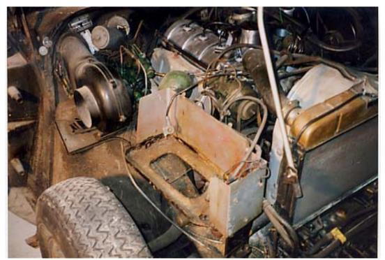
Work starts on stripping out the engine bay. On the '66 RHD Pallas, the battery is carried on the offside. The battery box was found to be heavily corroded and was largely rebuilt. When re-building the car, a battery mat (available from Frost) was used underneath the battery tray itself. This mat will absorb and neutralise any future acid spill.
