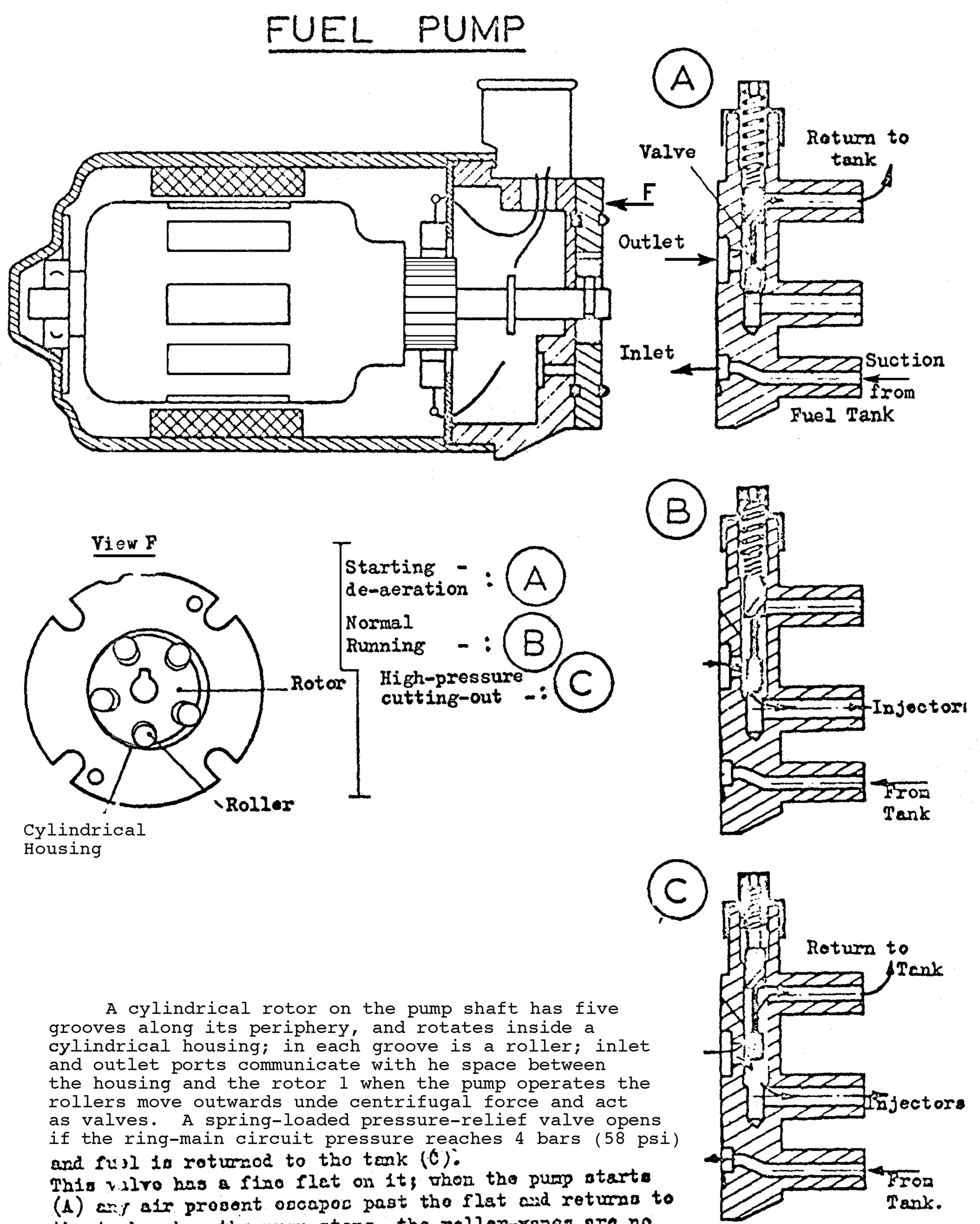
the trik; when the pump stops, the roller-venes are no longer held out by contrifugal force; fuel escapes from the ring-main along this flat until the line-pressure falls to 1.3 Kg/or2 (182 psi) at which point the valve closes. The pump is full of fuel at all times, eliminating shaft-leals and the friction they would introduce. The pump output of approx. 13 galls/hr exceeds the maximum requirements of the engine (92 galls/hr) and thus ensures that fuel circulates continuously.
