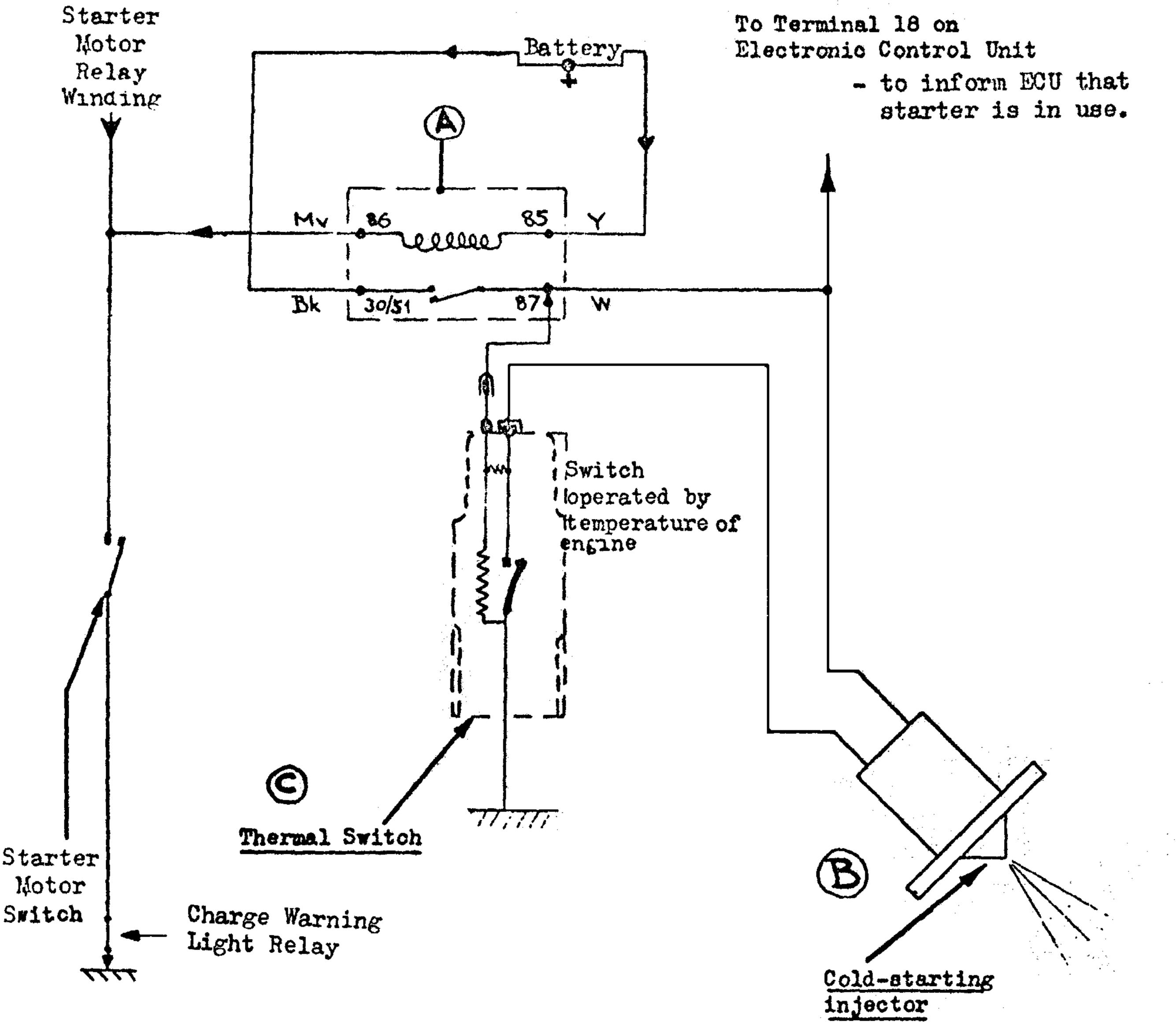
Relay, Impulse:- for cold starting injector, energised only when starter motor is in use.
