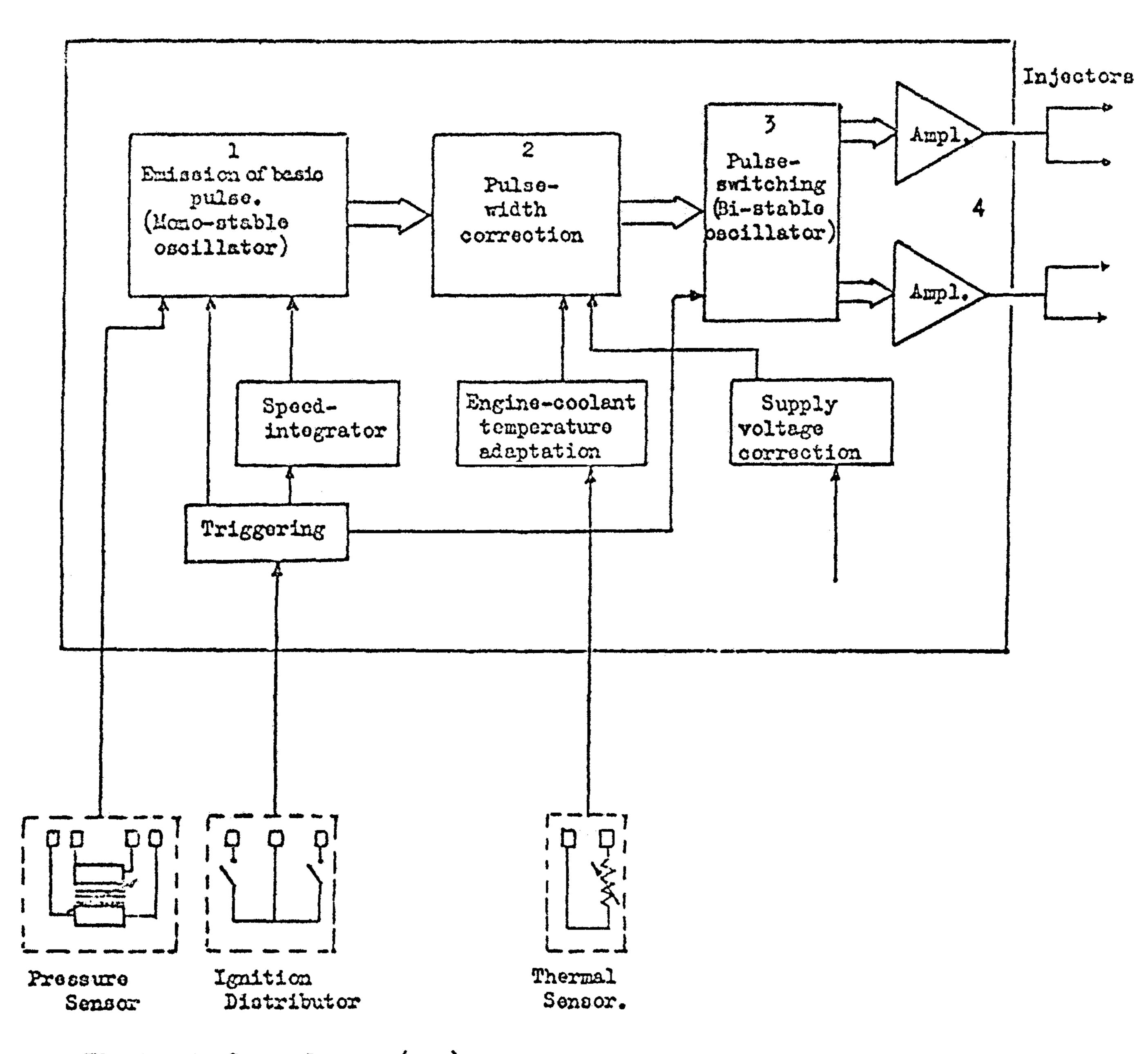
Electronic Control Unit (ECU):- receives signals from the various sensing clements, creates pulses, corrects the pulse-width, directs them to one cr other pair of injectors, amplifying them to operate the injector colenoids at 3 volts. Also controls operation of Fuel Pump when engine starts and stops.
