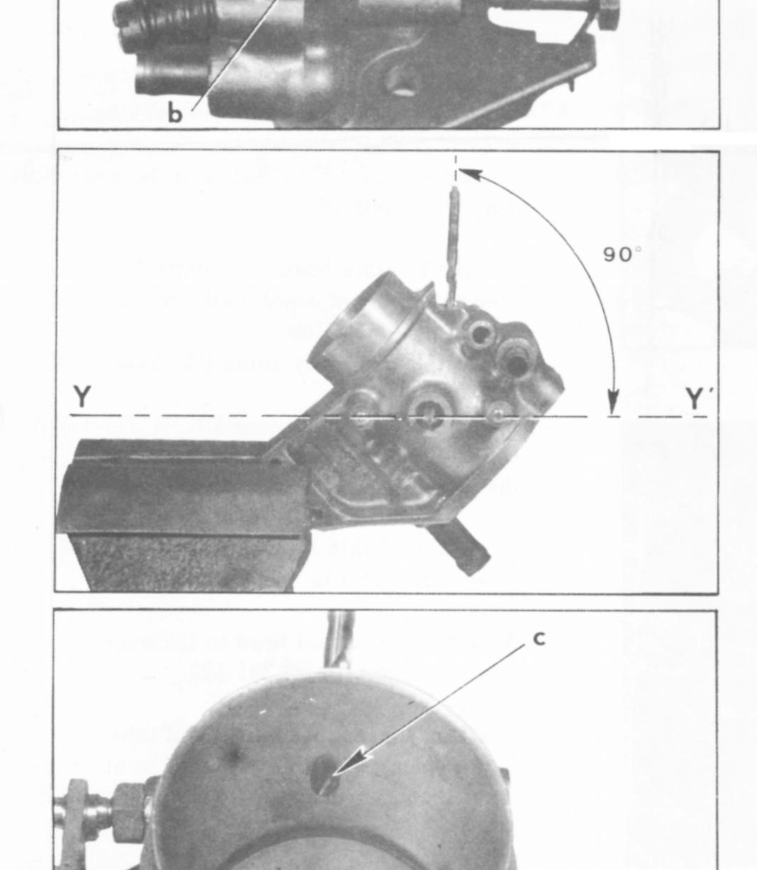
This hole must come out onto the idling air tube (seen through hole «c»)
