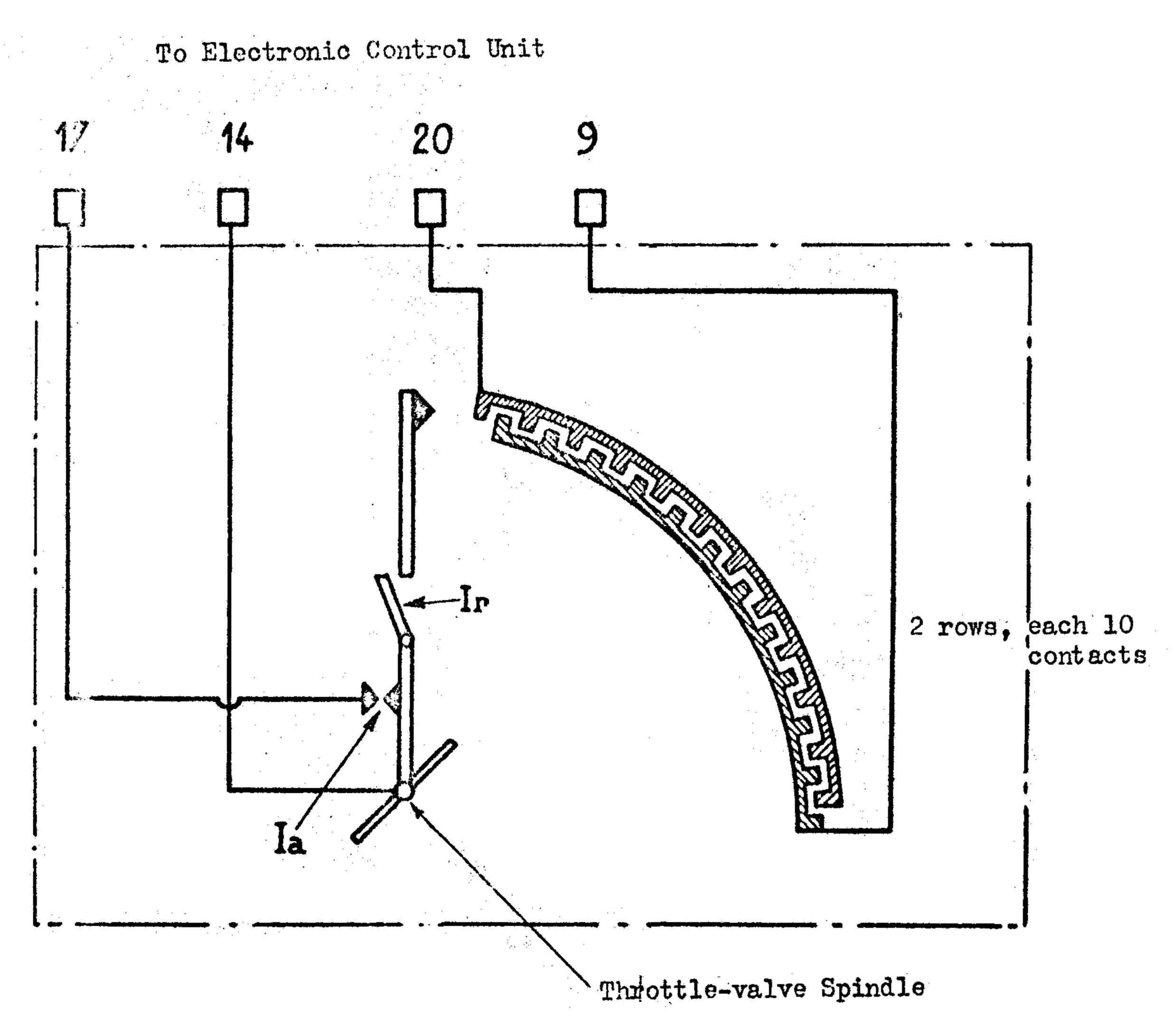
Throttle Spindle Switch:-
