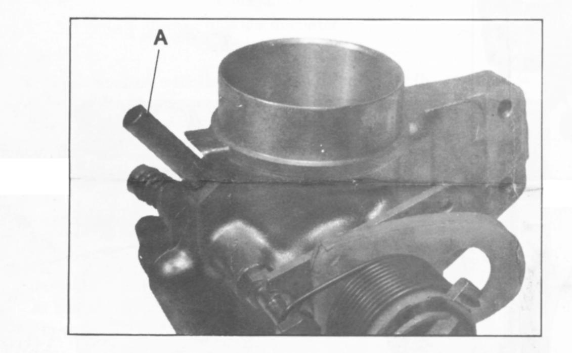
g) Spray the activator LOCQUIC-T in the hole and allow to dry completely. Smear the edges of the hole and the bevel end of tube A with LOCTITE N° GX. 01. 460. 01 A Place the tube in the hole and position it so that the bevel end blocks hole «c» Allow to dry for approximately one bour
