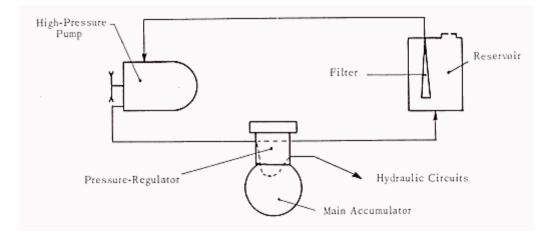
• To ensure the correct operation of all the hydraulic units a certain minimum pressure must be maintained in their supply circuits.
