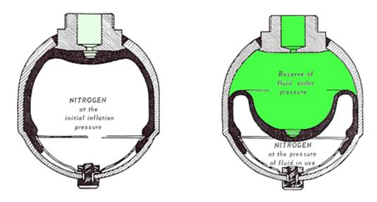
• This condition continues until the initial inflation pressure of the accumulator is reached. Then the diaphragm comes into contact with the shell of the accumulator.
