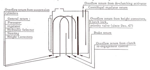
b) Reservoir for vehicles wich manual control of gearchange and clutch.
