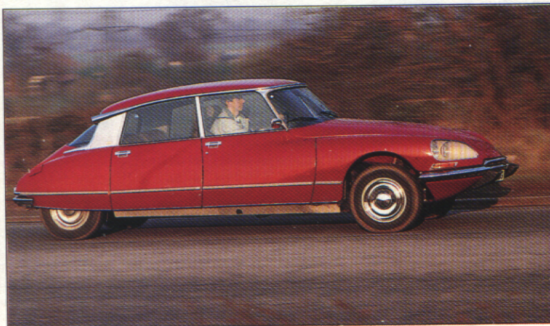
Fluid-based suspension and long wheelbase give the big Citroëns an unrivalled ride
