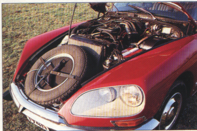
1974 DS 23 uses a 2347cc fuel injected four-cylinder engine
